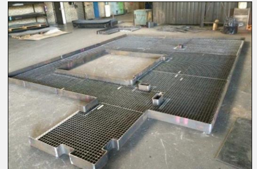
Flooring released for corrosion protection
