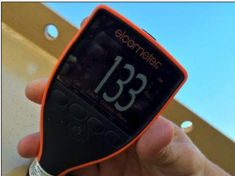
Painting DFT inspection and quality checks
