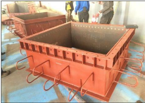
Secondary crusher cast-in chutes release for delivery to site
